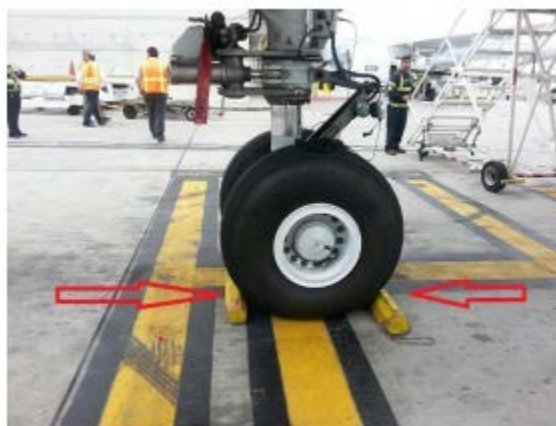
Figure 1: Proper Placement of Chocks; both in front of and behind main wheels
