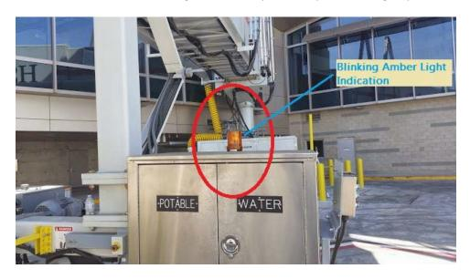
If the amber beacon is on, either the nozzle coupling is not connected to the air Gap coupling or the nozzle ball valve is in the closed position.
